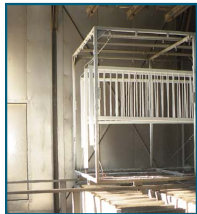
The owners invested in an energy-efficient batch oven with an enlarged opening to accommodate oversized parts.
